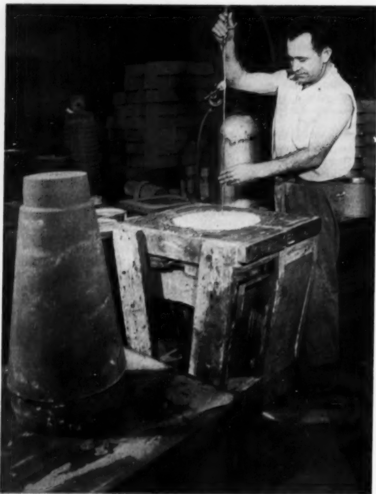
Cooper Alloy Corp., Hillside, N. J., has introduced the CO 2 process into its stainless steel foundry. The 200 lb core shown here was previously made in halves with an oil sand. Each half was baked for 8 hours. Now, gassing in two locations for 20 to 30 seconds at 30 psi hardens the core. Coremaking time is reduced from 75 to 25 minutes and rodding is reduced 60 per cent
